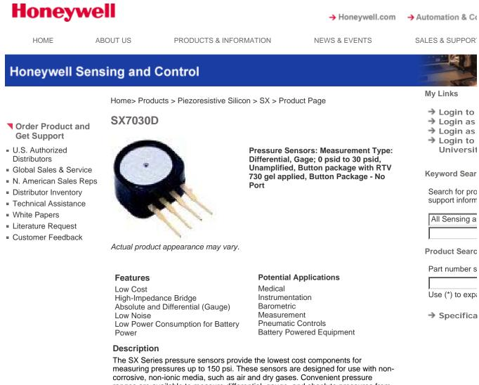
ranges are available to measure differential, gauge, and absolute pressures from 0 psi to 1 psi (SX01) up to 0 psi to 150 psi (SX150). The Absolute (A) devices have an internal vacuum reference and an output
